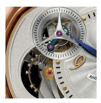
Most notably, positioned at 10 o'clock, a three-arm bridge spans an aperture, with the unusual blued seconds hand moving in discrete one-second steps beneath. It is the combination of the unconventionally shaped seconds hand, star-shaped wheel and spiral spring which provide an indication that the movement within the Sauterelle is atypical.
