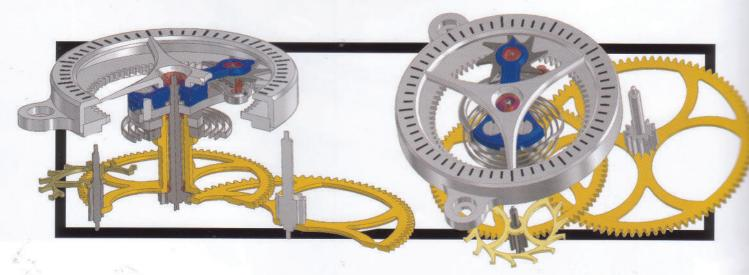
dial. The spokes of the centre, and the subsequent wheels, repeat the butterfly motive. The centre wheel is also called the 2nd wheel, and using this terminology we arrive at the 4th wheel which turns once a minute and is also called the 'seconds wheel'. It carries the remontoire and the jumping seconds hand. There can be no doubt that Strehler merited the 2013 Gaïa Prize for creative horology.
